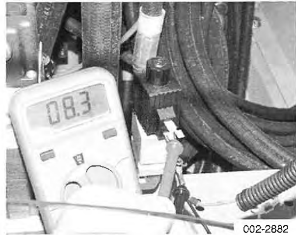
Testing solenoid coil resistance
