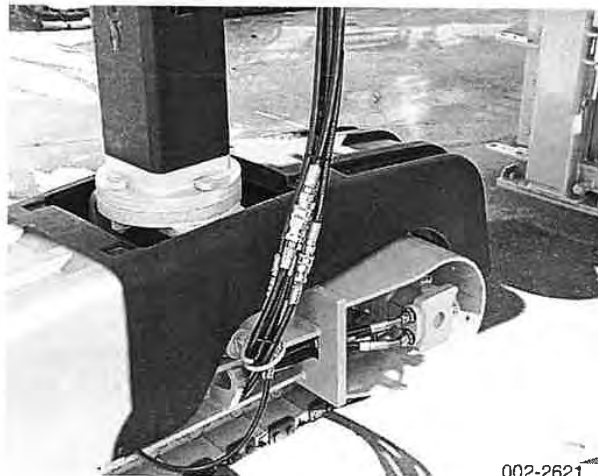
Tighten track yoke bolts
