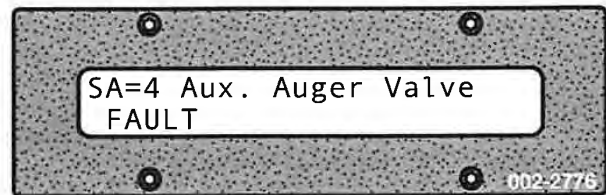
Auxiliary auger valve fault display
