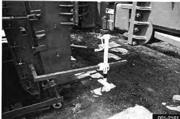
Attach sensor mount arm
