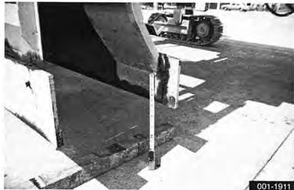
Adjusting rear sideplates
