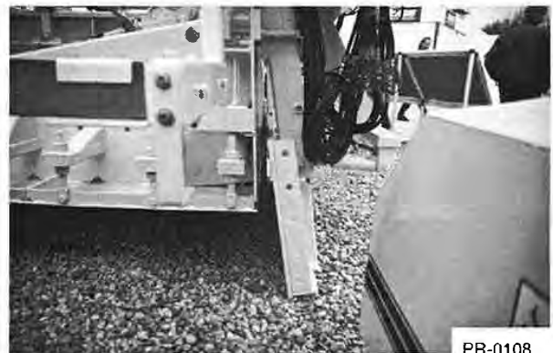
Vertical hinged sideplate swing clamps
