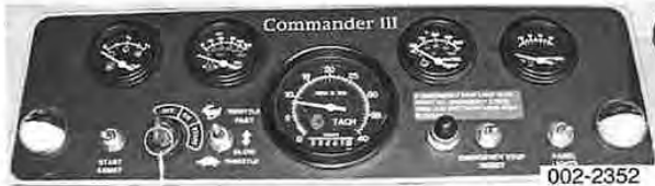
Reset the emergency stop light
