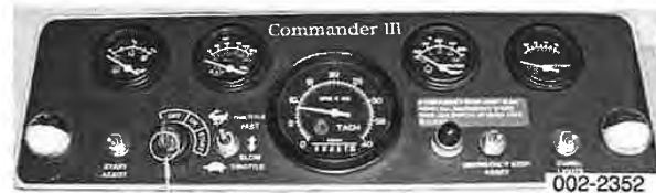
Reset the emergency stop light
