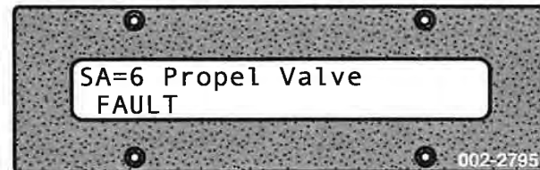
Propel valve fault display
