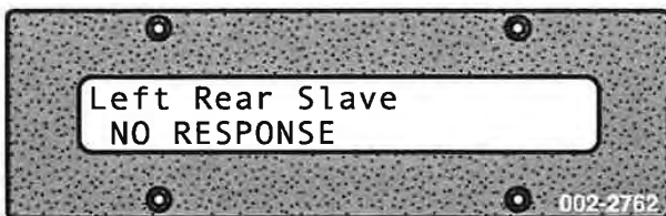
S2X controller failure
