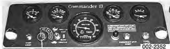
Reset the emergency stop light
