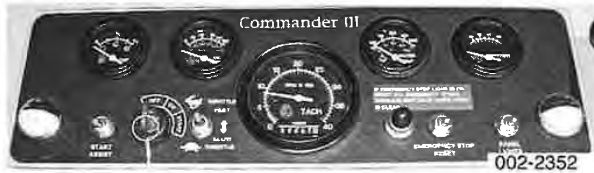
Reset the emergency stop light
