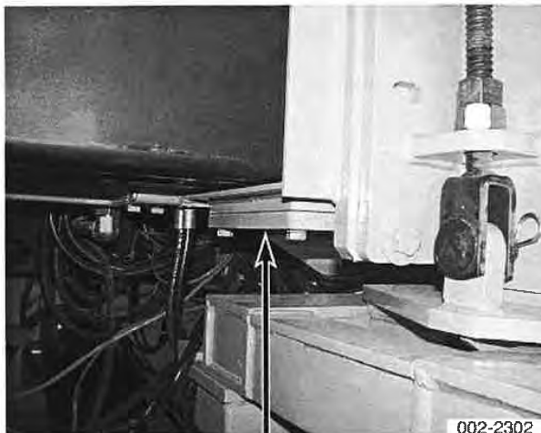
Tension right front leg wear pad
