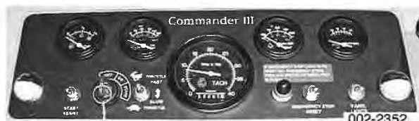
Reset the emergency stop light
