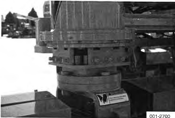
Tension right front leg wear pad
