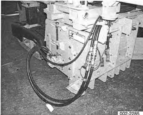
Check for defective quick couplers
