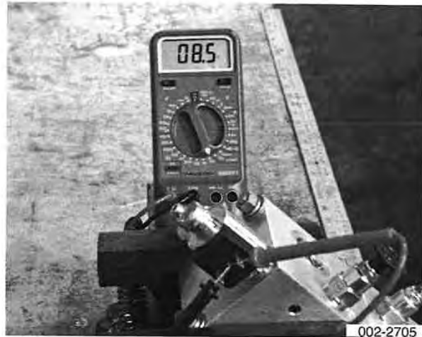
Vibrator solenoid coil resistance
