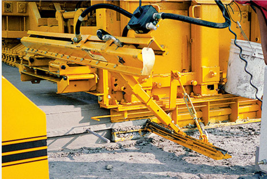
Male keyway with side bar inserter (SBI).
