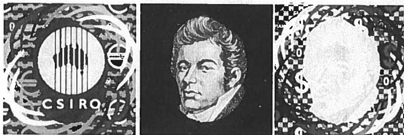
Figure 5. Example of an Exelgram OVD demonstrating both i) a switching between two images (CSIRO logo and face of early Governor John MacArthur) and ii) a positive tone to negative tone image change as observed at three different angles of view.
