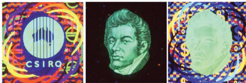
Fig. 7.12. Exelgram OVD showing two-channel switching and portraiture effects
