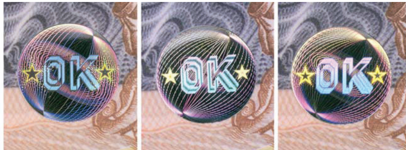
Fig. 7.3. Characteristic opto-kinetic Kinegram OVD effects at three angles of view
