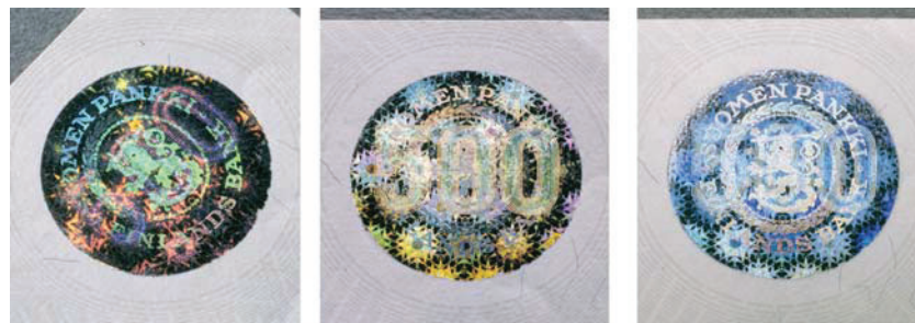
Fig. 7.4(a). Optical behaviour of the Kinegram on Finnish 500 mark banknote
