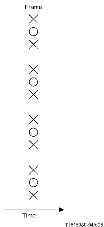
Figure 6-4 – Vertical and temporal positions of samples in a progressive frame
