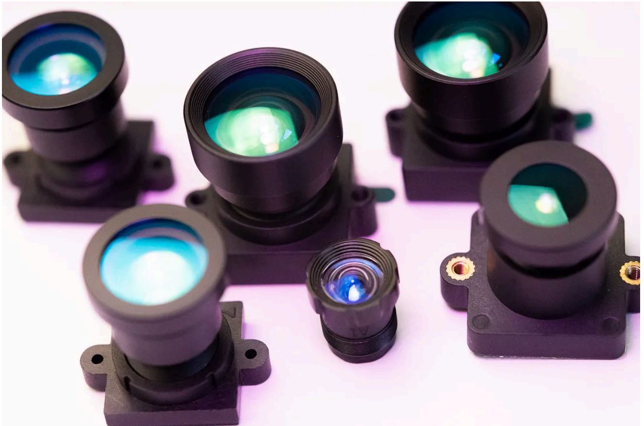
Time-of-Flight specific lenses from various manufacturers. The green or blue hue is from the specific anti-reflective lens coating to reduce lens flare and therefore multipath interference.
