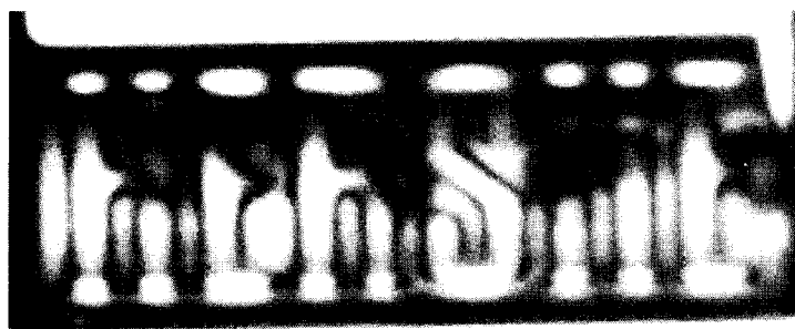
A picture of a candy bar made using T-rays. The nuts, which were hidden beneath the chocolate, are visible as a result of refraction. (Photo courtesy V. Rudd, Picometrix, Inc.)
