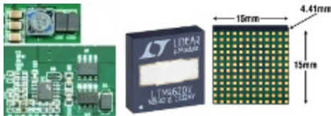
Zoom image: Figure 17. A 3-Phase, Single VO High Current Buck Converter Using the LTC3829
