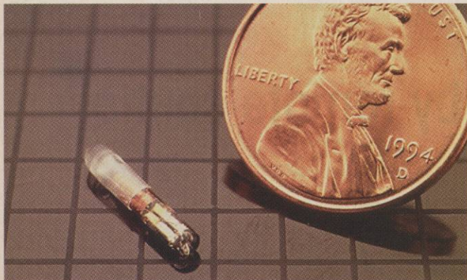
Despite its miniscule size, Digital Angel's Bio-Thermo microchip contains a temperature sensor and ID information on the animals in which it is implanted.
