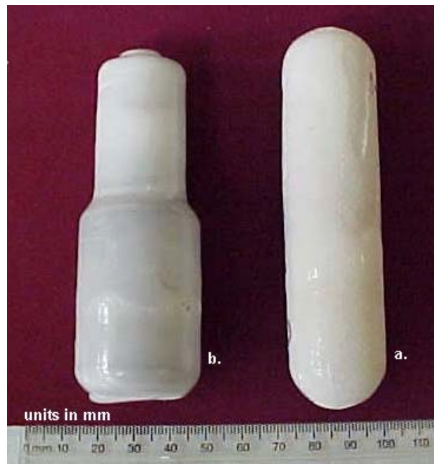
Figure 4. Cattle transmitters: a. Original transmitter(1), b. Improved transmitter (2)
