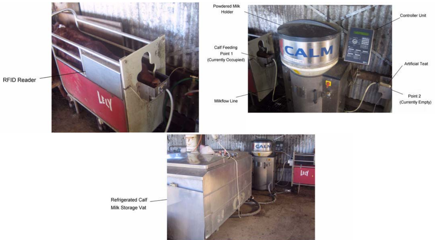
Exhibit 5.8 Calf Feeding Equipment – Top Left: Calf suckling milk from artificial teat; Top Right: Calf feeder unit; Bottom Centre: Refrigerated vat for holding milk to feed calves.
