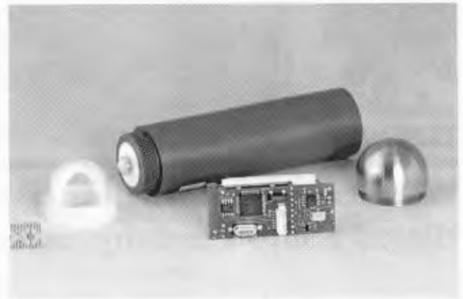
Fig. 2 – Disassembled bolus, in use the system is sealed.
