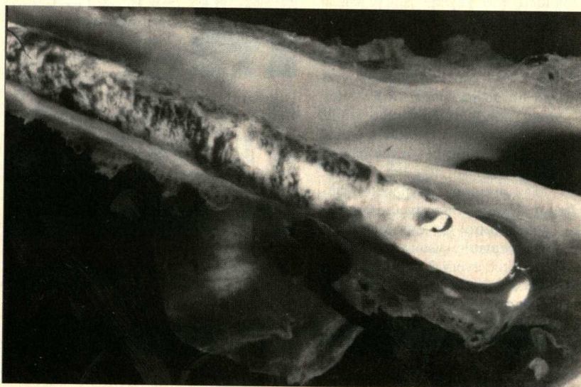
10. Explanted intravascular catheter with a sensor at the tip showing fouling of the surface (courtesy of Professor J Feijen, Twente University of Technology, Enschede, The Netherlands).
