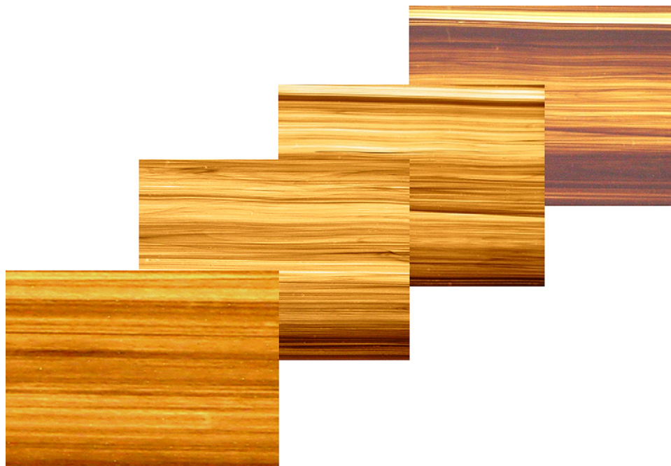
Figure 22.12 Realistic simulated wood grain patterns formed controllably in extruded film. Because chaotic motion underpins the process used to form them, each extrusion can have a unique pattern if desired. Stone-like and abstract patterning can also be imparted.
