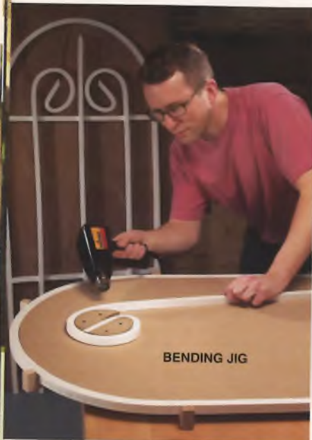
Bending thin strips of plastic lumber is very easy. With a heat gun, a bending jig and a little creativity, you can open up a world of possibilities.
