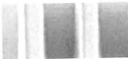
Figure 35. Portion of an SEM image of two parallel lines of photoresist on a silicon wafer and the signal profile across them. The relationship between the physical profile and the signal depends upon the slope and roughness of the sides of the lines, the composition of the material, the electron accelerating voltage used, and the electron detector used.
