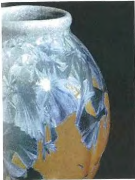
Figure 2. Photograph of a glaze covering a ceramic pot. The glaze flows down the surface in a molten state and solidifies to an amorphous glass under the forces of surface tension. Subsequently, the atoms rearrange themselves to form crystals which nucleate and grow in the glaze, producing visually interesting patterns and also modifying the surface geometry.
