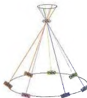
Figure 41. Tilting the sample in a conical pattern produces a series of projections used for reconstruction in transmission electron microscopy. The spacing along the cone trace is generally not uniform.
