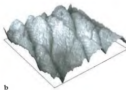
Figure 7. Scanned stylus image of a plastic replica of human skin: (a) grey-scale representation of the elevation data; (b) photorealistic visualization of the surface.
