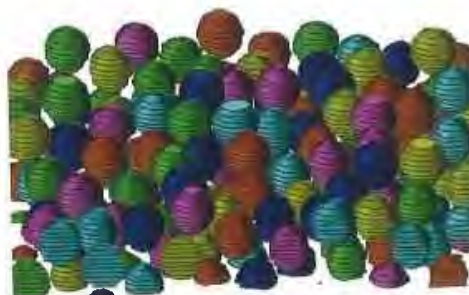
Figure 69. Rendered surface image of spherical particles from tomographic reconstruction (see Chapter 11, Figure 51 ) created by interpolating surface tiles between the slices shown in Figure 23 , and assigning arbitrary colors to each feature.
