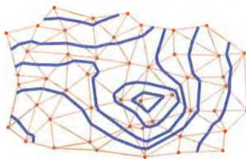
Figure 9. Drawing contour lines (iso elevation lines) on the triangular facets joining an arbitrary arrangement of points with elevations that have been determined by stereoscopy.
