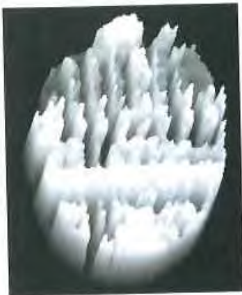
Figure 54. Isometric display of elevation data within a volume. The height of the surface having the maximum concentration on Si in the SIMS voxel array.
