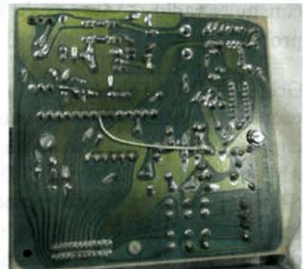
An example of hand-drawn etched traces on a PCB
