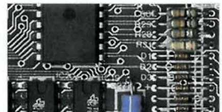
Part of a 1984 Sinclair ZX Spectrum computer board, a printed circuit board, showing the conductive traces, the through-hole paths to the other surface, and some electronic components mounted using through-hole mounting
