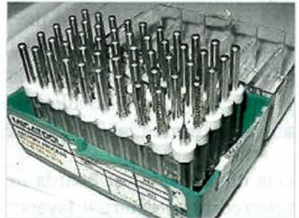
A box of drill bits used for making holes in printed circuit boards. While tungsten-carbide bits are very hard, they eventually wear out or break. Drilling is a considerable part of the cost of a through-hole printed circuit board.
