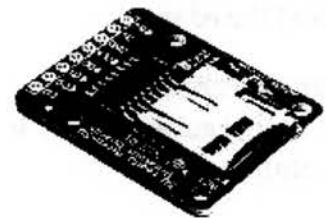
This breakout board allows an SD card's pins to be accessed easily while still allowing the card to be hot-swapped.
