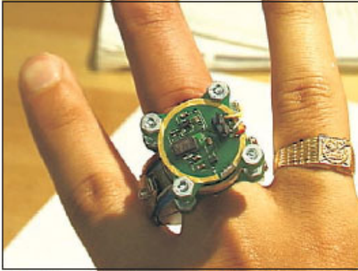
Fig. 9. First prototype ring sensor with RF transmitter powered by a coin-size cell battery.
