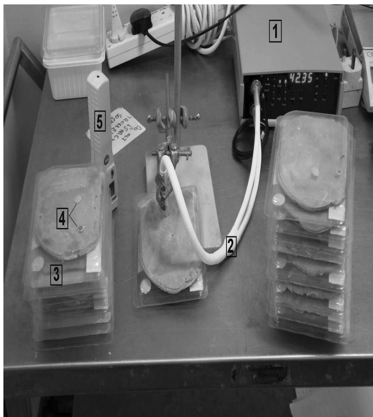
Figure 3.4 Use of platinum fluorescent-based disposable oxygen sensors in MAP packed sliced ham (number 4 in figure indicating as part of this mail).
