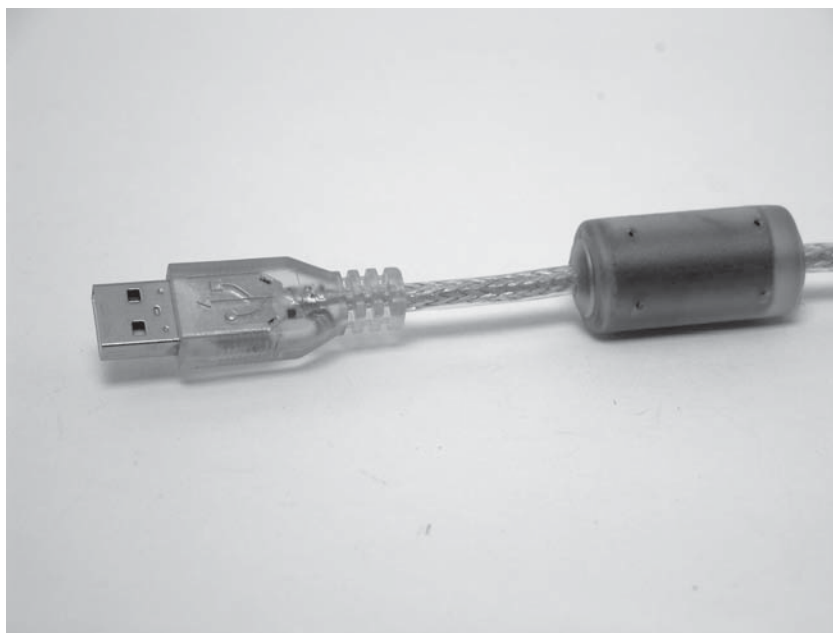
FIGURE 5-32. Ferrite core used on a USB cable to suppress radiated emissions.
