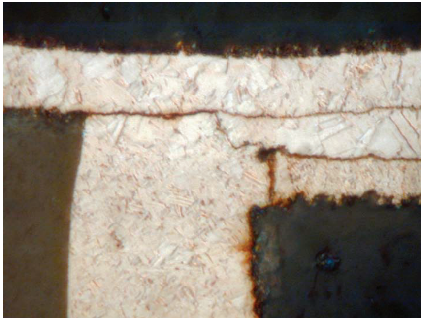
Figure 3: Photo showing wrap crack.
