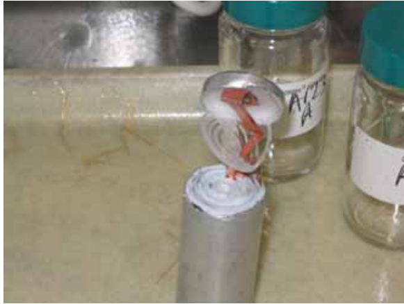
Open from the anode side
