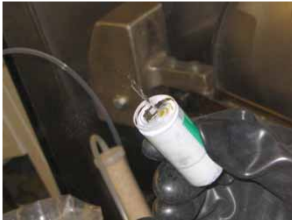
Cathode side of the jelly roll
