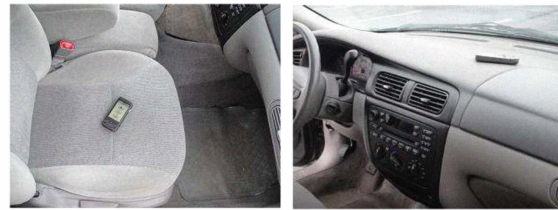
Fig. 5. The G1 phone is put on the front seat or the dashboard of the vehicle during drunk driving detection.
