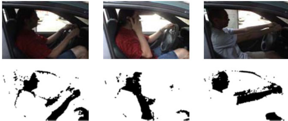
Figure 3: It is taken from the paper “Driver Activity Monitoring through Supervised and Unsupervised Learning” and shows skin color detection (bottom row) on various images (top). Skin color is indicated in black. The results are post-processed by a sequence of morphological erosions and dilations.
