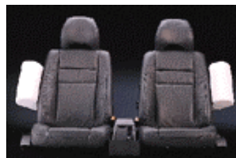
Figure 13 Side airbags in seat frames [64].
