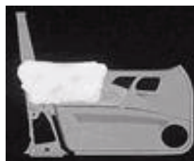
Figure 12 Side airbag in door panels [64].
