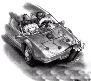
Figure 1 Three mechanical sensor system [62].
