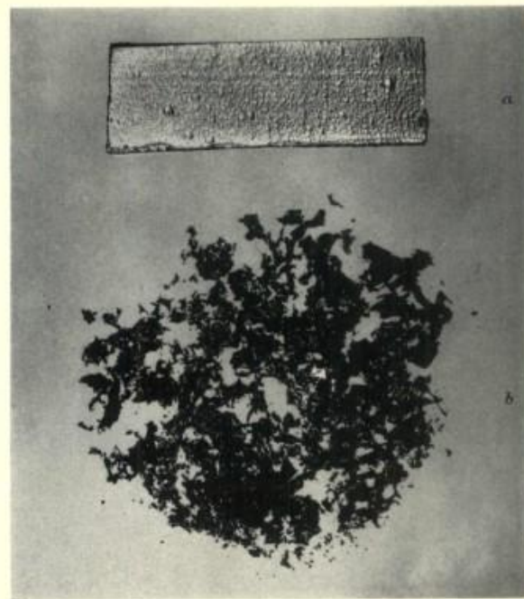
FIGURE 11. ( a ) Specimen of 'as-deposited' type A pyrolytic graphite. ( b ) Product after detonative 'stress-annealing'.
