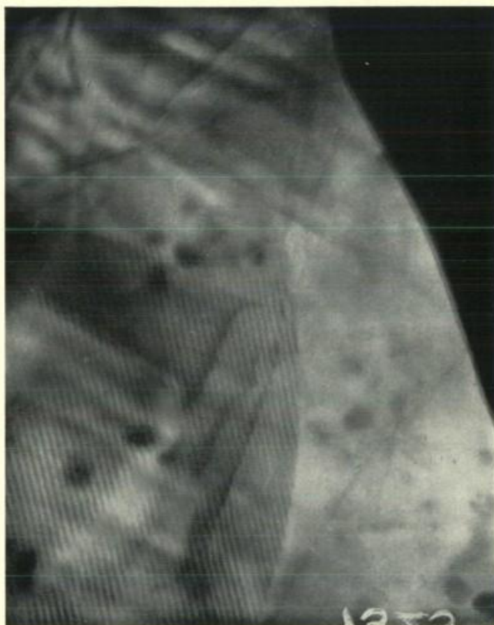
FIGURE 8. Electron micrograph of type B graphite showing Moiré fringe patterns.
