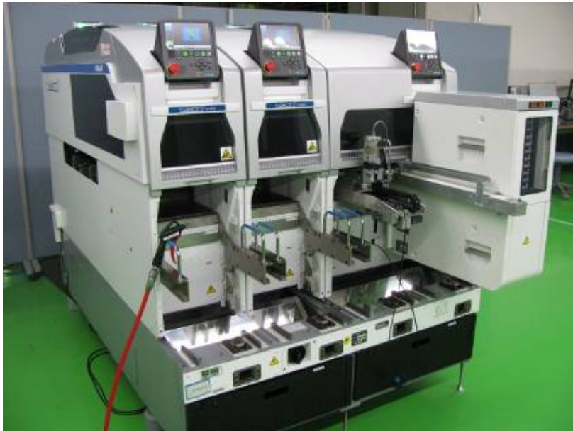
Surface Mounter: Fuji NXT
