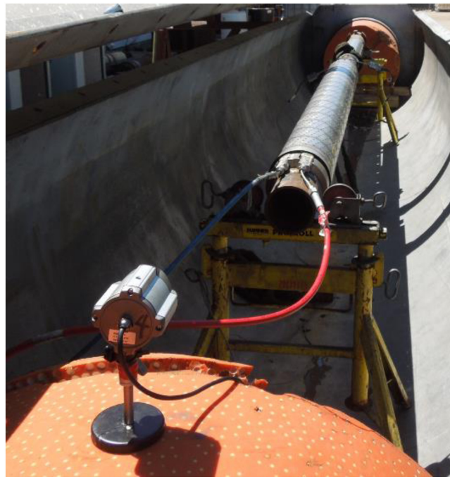
Figure 22—Image showing burst pressure test setup
