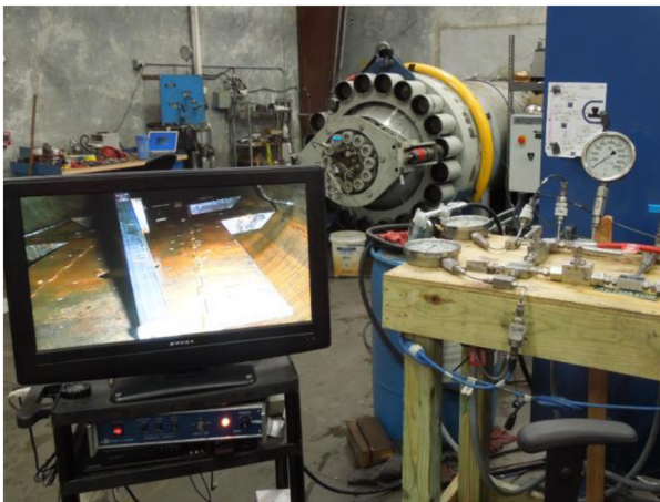
Figure 24—Image showing collapse pressure test setup
