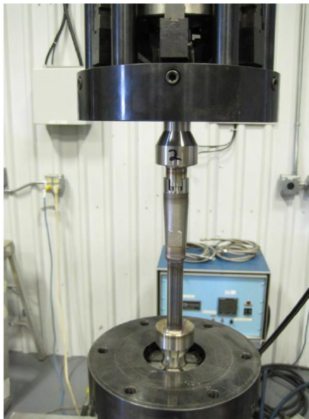
Figure 33—Setup for the jumper tubing connection tensile test.
