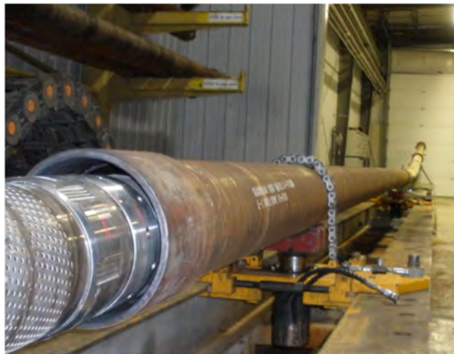
Figure 19—The dog leg (bending) test setup is shown on this image.
