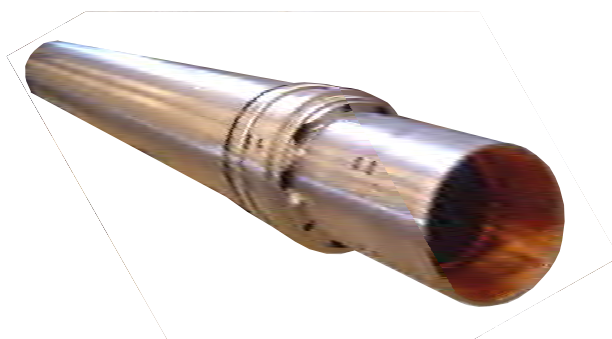
Fig. 3. Shunt System Manifold Box-End (without outer sleeve)
