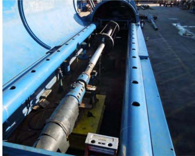
Figure 14—The fixed shroud tension test sample placed into a test bay with a loading frame.
