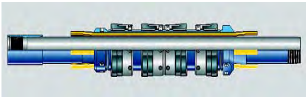
Figure 8 – Multi-zone packer. Note the beveled gauge ring close to the pin end.
