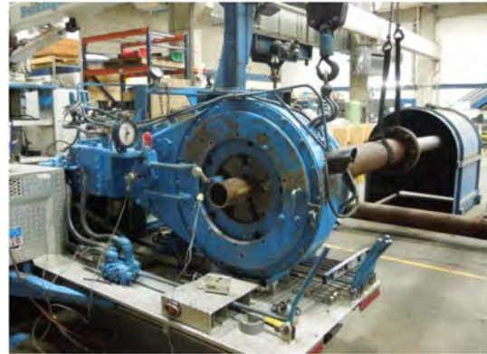
Figure 16—Outer shroud torque test setup.
