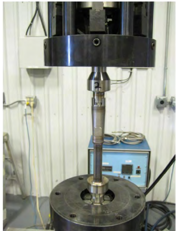
Figure 33—Setup for the jumper tubing connection tensile test.
