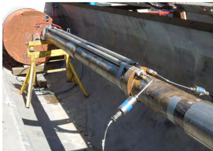
Figure 31—Test setup for the jumper tube burst pressure test, showing the test when sliding shroud was not used.
