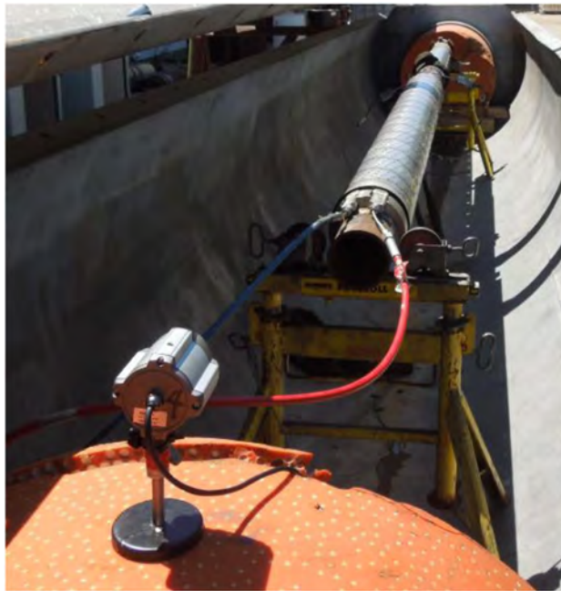
Figure 22—Image showing burst pressure test setup
