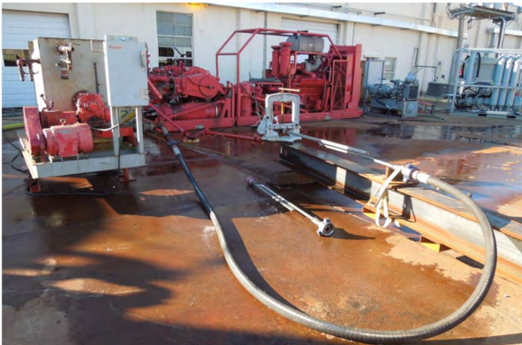
Figure 37—Image showing the typical erosion test setup.
