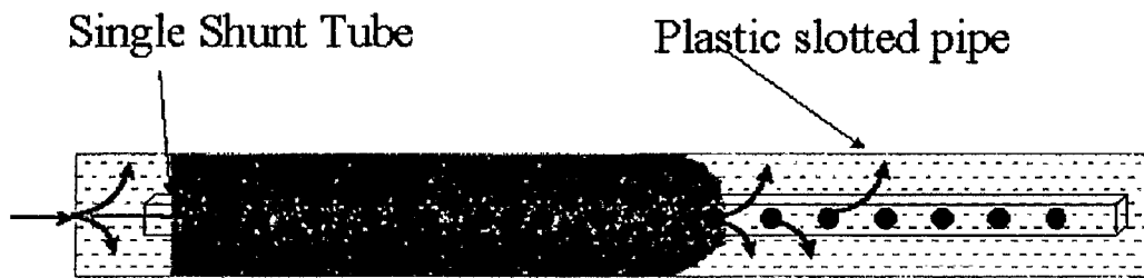
Fig. 3 -Surface tests performed with shunts in horizontal mode and slotted plastic pipe used as the formation with high leak-off. Flowed into the the liner and then down the shunt tube. Resulted in 500 ft completely packed with one shunt.
