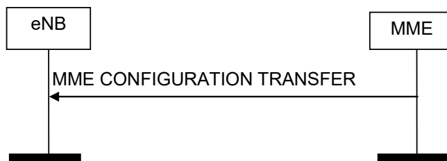
Figure 8.16.2.1-1: MME Configuration Transfer procedure. Successful operation.
