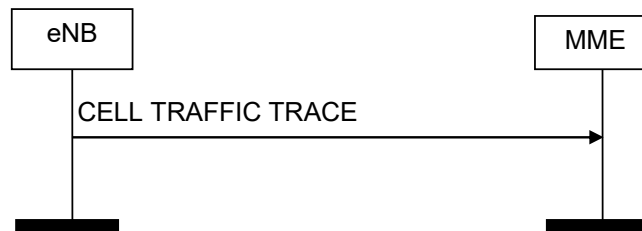
Figure 8.10.4.2-1: Cell Traffic Trace procedure. Successful operation.
