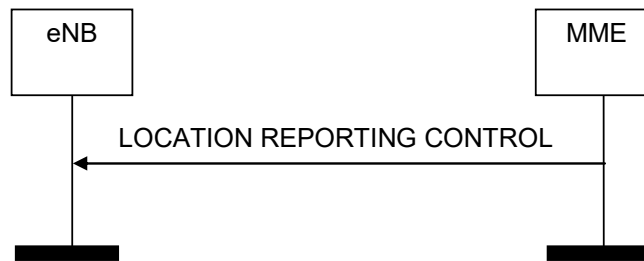
Figure 8.11.1.2-1: Location Reporting Control procedure. Successful operation.
