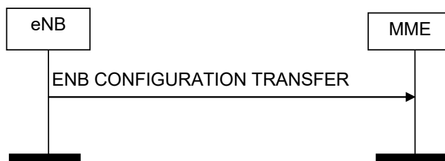
Figure 8.15.2.1-1: eNB Configuration Transfer procedure. Successful operation.
