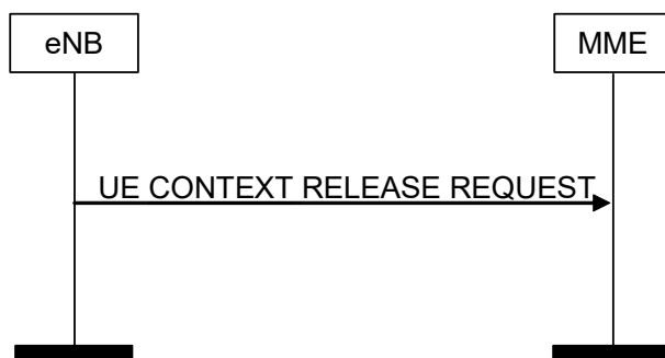
Figure 8.3.2.2-1: UE Context Release Request procedure. Successful operation.
