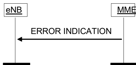
Figure 8.7.2.2-1: Error Indication procedure, MME originated. Successful operation.
