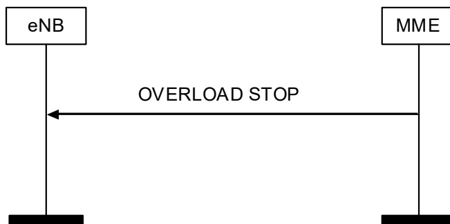
Figure 8.7.7.2.-1: Overload Stop procedure
