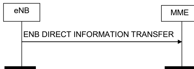
Figure 8.13.1.2-1: ENB Direct Information Transfer procedure. Successful operation.
