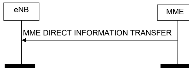
Figure 8.14.1.2-1: MME Direct Information Transfer procedure. Successful operation.
