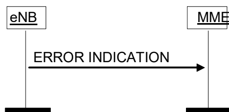
Figure 8.7.2.2-2: Error Indication procedure, eNB originated. Successful operation.
