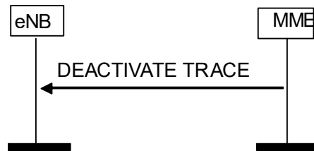
Figure 8.10.3.2-1: Deactivate Trace procedure. Successful operation.
