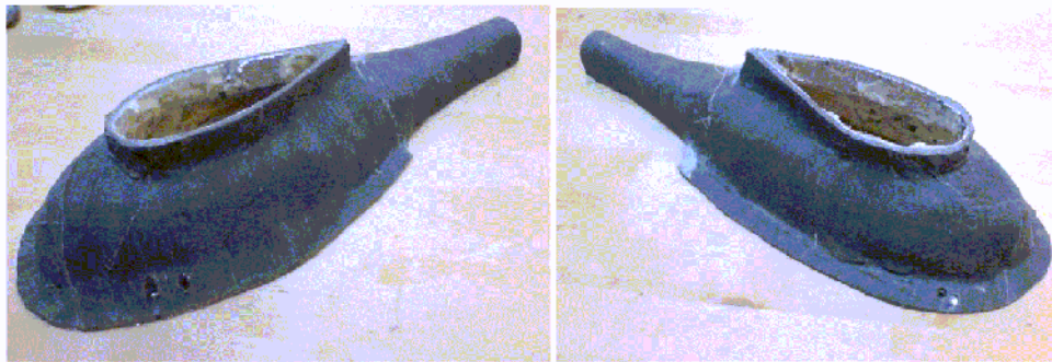
Figure 3. Results of test lamination.
