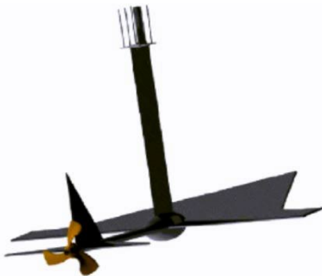
Figure. 9. Illustration of Evolo's underwater body
