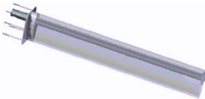
Figure. 10. Illustration of Evolo's strut
