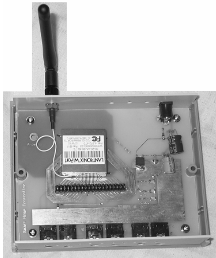
Figure 6: Wiport Controller Box
