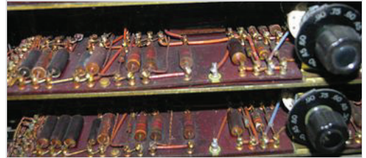
Point-to-point construction of military radio equipment
