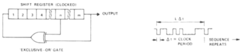
FIGURE 1 PSEUDORANDOM SEQUENCE GENERATOR USING SHIFT REGISTERS.
