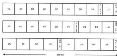
Figure 9.14 Possible implementations of an SDMT frame for different upstream and downstream bit-rate ratios.
