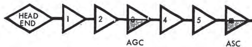
B. Generalized Trunk System with AGC & ASC Truck Amps.
