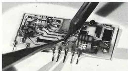
Fig. 4 Soldering through a polyurethane conformal coating on a ceramic printed-circuit assembly.
