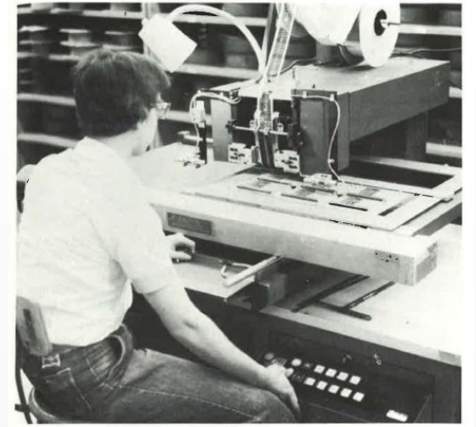
Fig. 9-3. Computer-controlled automatic insertion machine. (Courtesy Computevision Corp., Bedford, Mass.)
