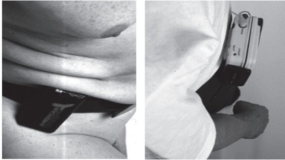
Figure 6. Single point attachment of a common pager or portable stereo is unstable and perceptually separate from the body.
