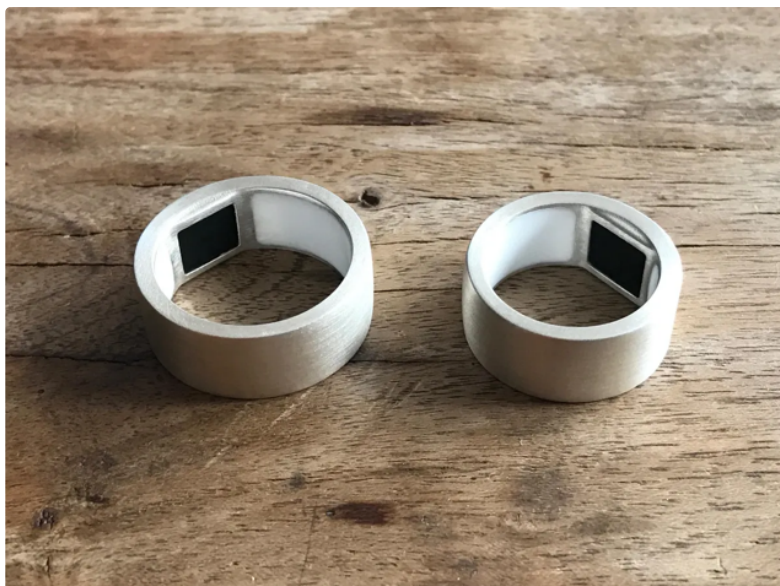
Token in two sizes. The fingerprint reader's on the inside.
