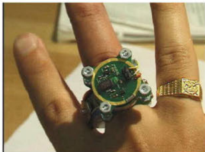
Figure 2: Earlier design of PPG ring sensors
