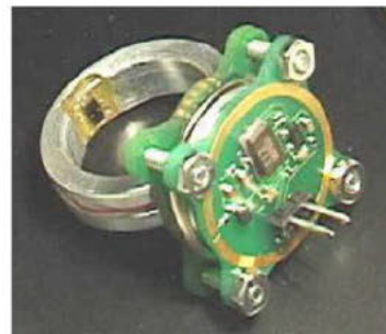
Figure 2: Earlier design of PPG ring sensors
