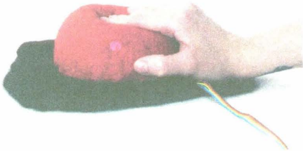
Figure 7-77. "Felt Pressure-Sensitive Button" by Lara Grant
