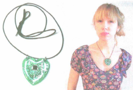
Figure 7-48: “Heart Spark” by Eric Boyd is a custom-designed printed circuit board necklace that receives a signal from a Polar heart rate monitor band and blinks in unison with the wearer’s heartbeat
