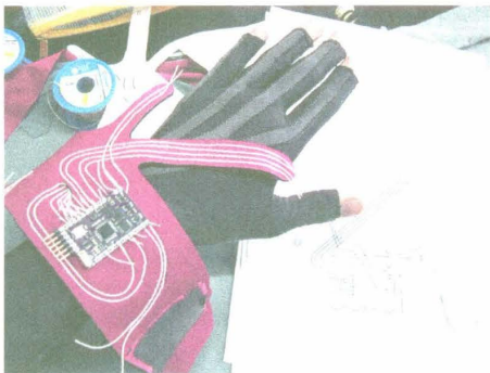
Figure 7-24 “The Gloves Project” uses flex sensors to create experimental gestural music; the project is developed by Rachel Freire, Imogen Heap, Seb Madgwick, Tom Mitchell, Hannah Perner Wilson, Kelly Snook, and Adam Stark (photograph by Hannah Perner Wilson)
