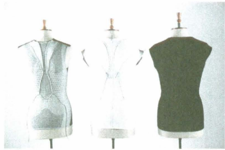
Figure 7-34. “Aeolia” by Sarah Kettley, with Tina Downes, Martha Glazzard, Nigel Marshall, and Karen Harrigan, explores the process of incorporating stretch sensors into garments through weaving, knitting, and embroidery techniques (photograph by Tina Downes and Catherine Northall)
