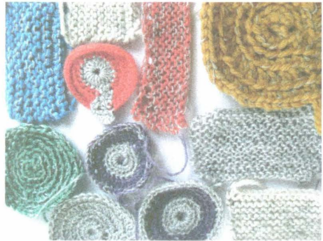
Figure 7-78. Knitted Pressure Sensors from How To Get What You Want
