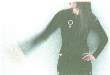
Figure 7-39. The accelerometer shirt by Leah Buechley uses accelerometer data to control the color of an RGB LED
