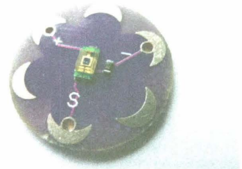
Figure 7-7. Closeup of LilyPad light sensor: note the resistor on the right as well as how the circuit board traces create a voltage divider circuit
