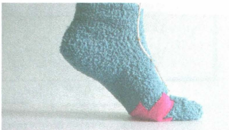
Figure 7-29. When pressure is applied to the ball of the foot the change in sensor data can be read by the microcontroller
