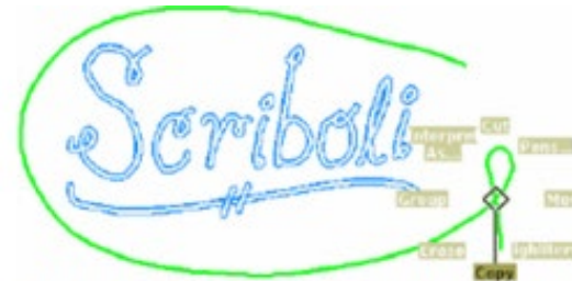
Fig. 1. Pigtail splits the user's gesture into a lasso, which here selects the ink, and a mark, which here chooses the Copy command from 8 possibilities.
