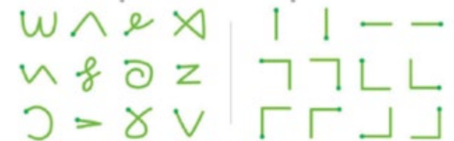
Figure 2. Free-form gestures (left) incl. pigtail [35], spiral [36], downward caret [17], Z [37], X [38], upward caret [38], "delete" [38], "squiggle" [17], and "redo" [28]. Mark-based gestures (right). Dots indicate start of each gesture.
