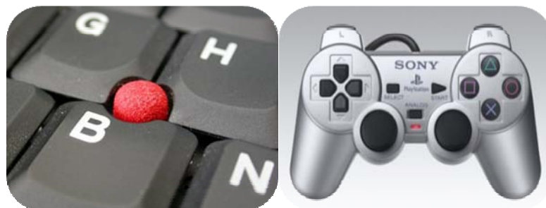
Figure 2-13: Examples of force sensing hardware. (Left) IBM's Trackpoint joystick. (Right) Sony's PS2 DualShock2 controller.
