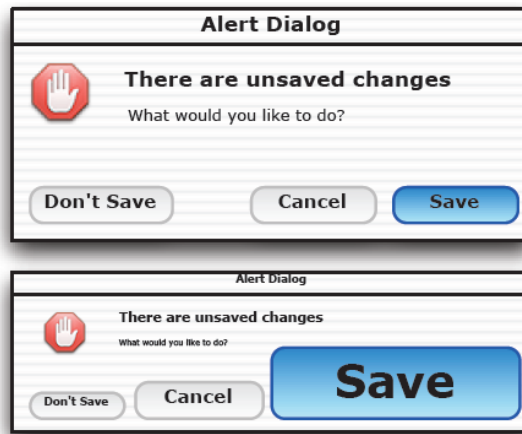
Figure 5-2: Example of a dialog window where its buttons are weighted according to their semantics. (Top) how the window looks visually. (Bottom) how the window looks in motor space –i.e., what it feels like when interacting with it.
