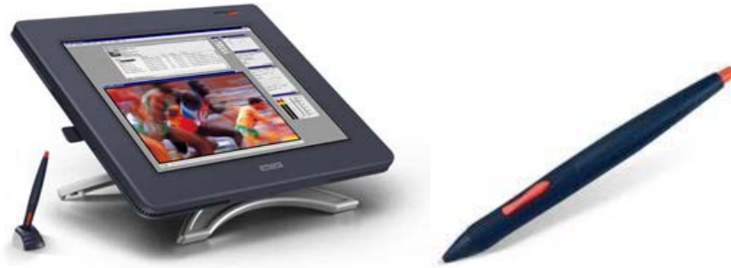
Figure 5-14: Wacom CintiQ interactive display with its accompanying pressure sensitive pen (enhanced detail on the right).
