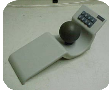
Figure 2-7: Spaceball used as a reference isometric device in Zhai's experiments
