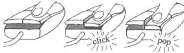
Figure 2-15: Pop-through mouse and an its three-state button.
