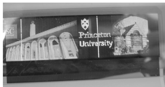
FIG. 3. Thin film encapsulated PHOLED display on 178 \mu m barrier coated PET. The encapsulation is comprised of five alternating pairs of Al 2 O 3 and polyacrylate; total thickness of the multilayer barrier stack is 5–7 \mu m. The 64 \times 240 display is passive matrix and capable of full motion video.
