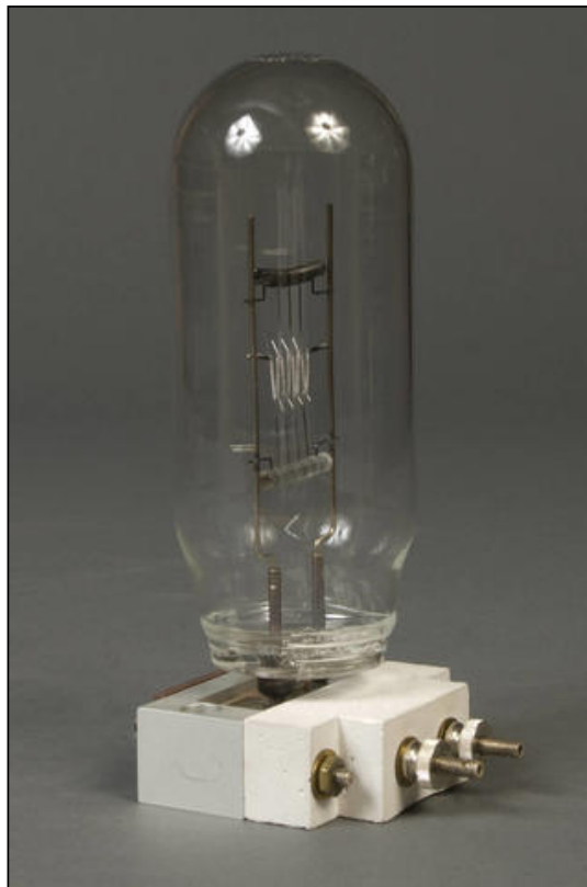
This artifact is a 500 Watt gas-filled incandescent lamp and was used as the luminous intensity standard in the 1970s.
