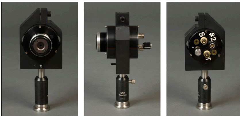
The 1979 redefinition of the candela made it possible to realize the unit using calibrated detectors of optical radiation. NIST implemented this technique in the early 1990s with this artifact, a silicon diode photodetector which included a filter that spectrally matched the accepted human visual response. This was the first use of a detector device to realize the candela for the United States, and was a
