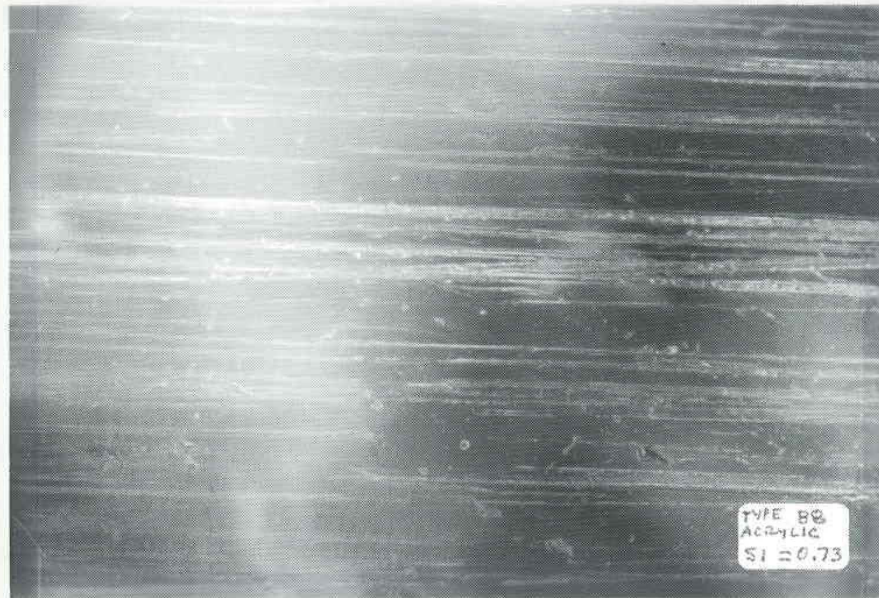
Figure 5-10. Photomicrograph of a plastic-faced Model 88 RPM subjected to 10 abrader passes.
