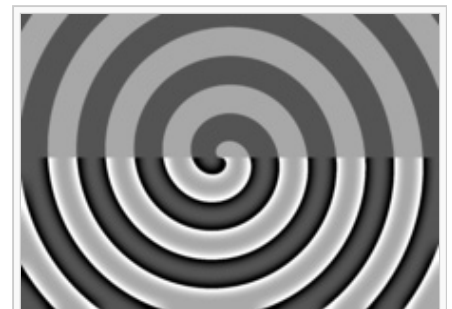
Another illustration, where overshoot caused by using unsharp masking to sharpen the image (bottom half) increases acutance.
