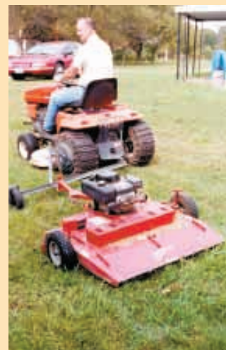
Roger Burgess had a hitch built that lets him pull a 40-in. Swisher mower - equipped with its own 8 hp Briggs & Stratton engine - behind his Ariens garden tractor.
