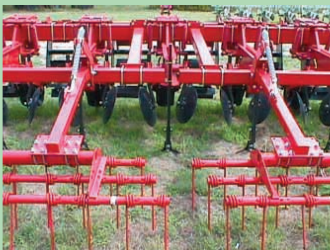
"It cuts and mixes residue into the soil as it rebuilds ridges," say Don and Kevin Ohlman, who came up with what they say is the ultimate, one-pass ridge-till tool.
