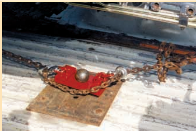
"Clamshell tie-down" consists of a couple pieces of 1/2-in. thick plate steel that fit on either side of the ball hitch and hook together with a lynch pin.
