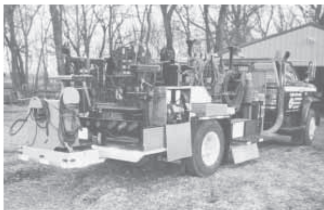
Brian Esser extended the frame of a 1981 2-ton Chevrolet truck to 30 ft. before installing his home-built utility bed.
