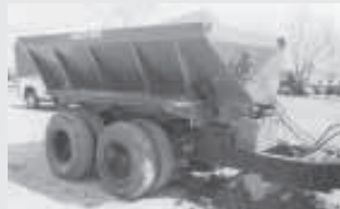
Cart's opening is in front so tractor driver can see material as it discharges.
