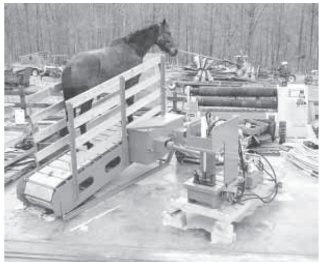
Here the pto powers an ice cream maker. Weaver also makes a hydraulic motor that runs off the pto. He has used that to power other equipment.
