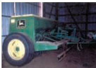
Drag consists simply of three 12-ft. sections of I-beam hanging from front of drill (left). Cox also uses drag on back of chisel plow (right).
