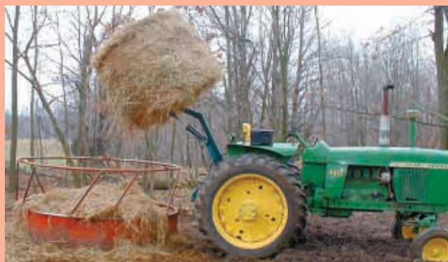
“My home-built, 3-pt. round bale spear lifts bales much higher than a conventional 3-pt. bale spear and can dump bales over a fence or into a feeder,” says Richard Hicks.
