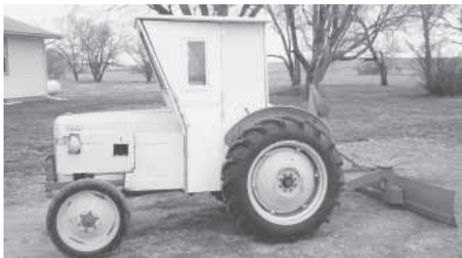
Using 3/4-in. plywood and metal sheeting, Ron Newton made a cab for his Ford 8N.
