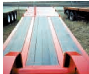
"Rumber" is made of ground-up scrap tires and recycled plastic. Here it was used to make a trailer floor.
