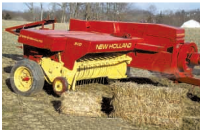
Scaled-down New Holland small square baler makes decorative 16 to 24-in. long bales that weigh just 6 to 8 lbs. Bale at right is a normal sized bale.
