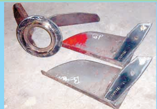
Modification requires bolting three pieces on front of rotor, just inside the feederhouse.
