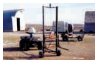
"It can raise loads up to 7 ft. high," says Mike Nordby about the 2-wheeled, electric-operated forklift he uses with his ATV.
