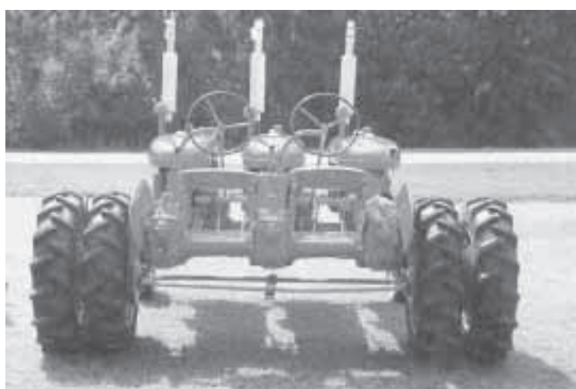
Tractor runs on one, two or three engines in any order. It has two steering wheels and two sets of clutch and brake pedals so Stewart can drive the tractor from either side.
