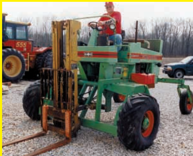
To make their Owatonna swather more useful during the off season, Tim and Tom Nelson mounted a 3-stage forklift mast on front. A hydraulic cylinder mounted underneath tilts frame forward and back.
