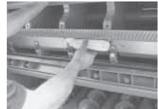
Kuchar filler plates reduce cylinder vibration by keeping dust out of cylinder.
