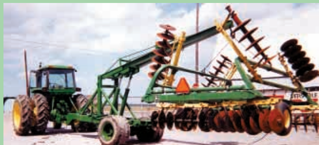
Loader tows behind a tractor and is hydraulically raised and lowered by an 18-ft. boom.
