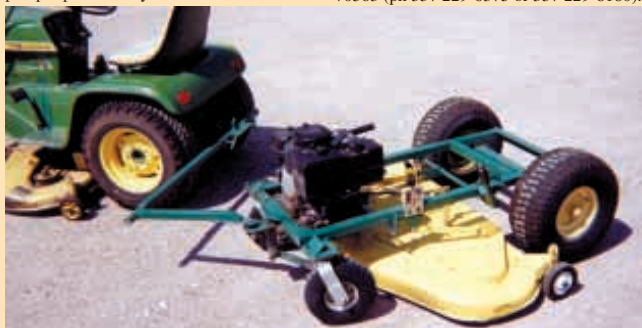
Richard Moore mounted the deck off a junked Deere 112 riding mower on a wheeled frame. He uses a Tecumseh 10 hp engine to power the trailing deck.
