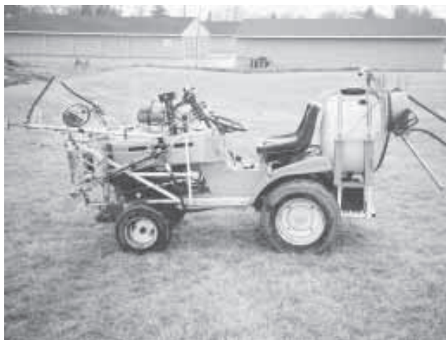
Gene Cafourek made this state-of-the-art mini spray rig by mounting a 16 1/2-ft. boom on front of his 18 hp garden tractor. He uses the sprayer to control weeds at three local cemeteries and on a half dozen local farmsteads.
