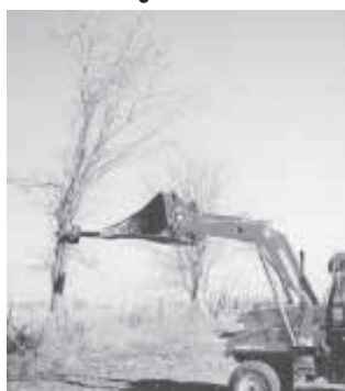
Tractor driver clamps the "claw" around tree while another person uses a chain saw to cut tree off.
