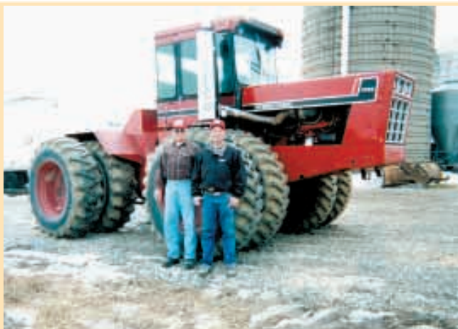
David and Ken Bense replaced the V-8 diesel engine on their 1985 IH 4786 4-WD tractor with a 6-cyl. Cummins 855 diesel engine out of an IH 4070 cab-over semi tractor. The tractor's original engine is high maintenance and parts for it are very expensive.
