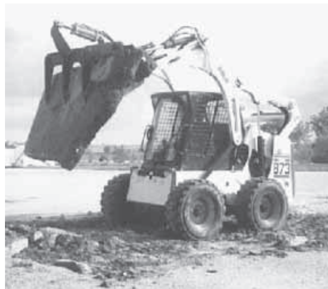
"It has super clamping power, which allows it to handle everything from concrete demolition and steel I-beams to big round bales," says Greg Gregory about his new heavy duty grapple fork for skid steer loaders.
