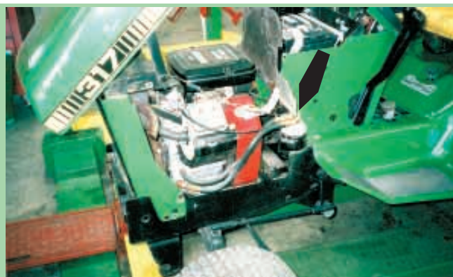
Deere 317 tractor originally had a Kohler 17 hp engine, which Kaczmarek replaced with a Vanguard 20 hp model. Note external oil filter relocation kit (arrow).
