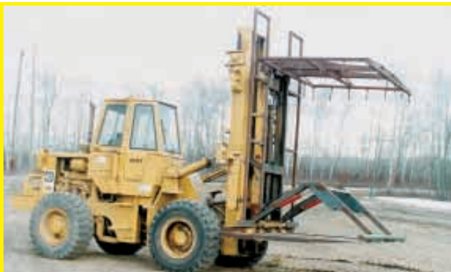
Home-built forklift device is used to handle 124-bale stacks. Extra top fork and a push-off bar help unload stacks.
