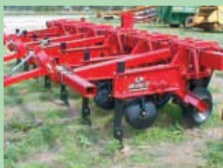
Tool has 6 or 8-blade choppers up front and ends with harrow sections on back.
