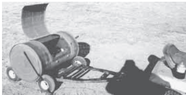
Home-built composter is made out of a 55-gal. drum and has an 18-in. door on one side.
