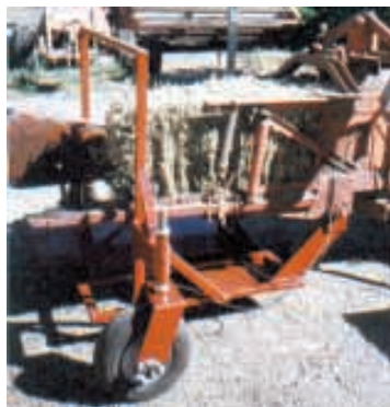
Tag-along bale scale rides on two small wheels directly behind bale chamber. In-cab monitor, above, tracks individual and cumulative weight.
