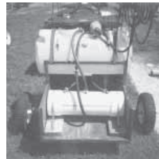
Spray tank mounts on an elevated cart and pulls chemical out of a reservoir that mounts in cart below the tank.
