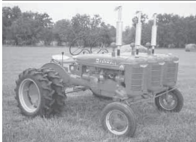
Dewitt Stewart of Bogalusa, La., mounted three Farmall A's together on a frame with a single front axle and a single set of rear dual tires.
