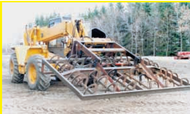
Ken Assenheimer stacks bales with a home-built self-leveling accumulator equipped with bale hooks that pull together, dosing the gap between bales.
