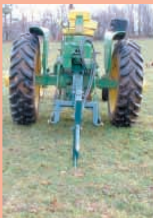
Boom holds bale perfectly level all the way to its stacking position.
