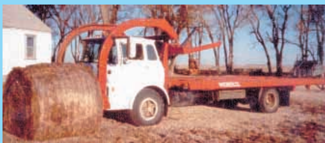
Bale-hauling truck designed by Richard and Dennis Weber is built around a 1972 Chevrolet C-50 cab-over truck. It can load up 10 big round bales on-the-go.
