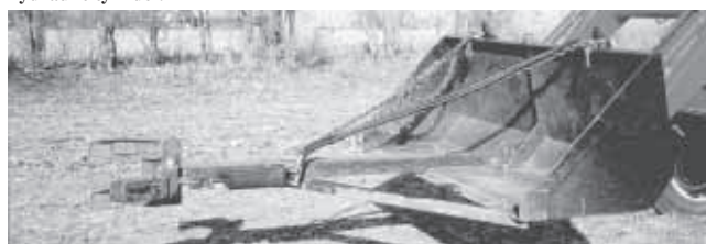
Unit is bolted to the end of a steel tube and extends about 7 ft. in front of loader bucket.
