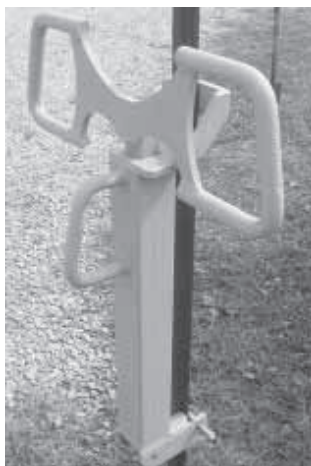
Post-Mate uses a pair of handles to both pound the post and also pull it out.
