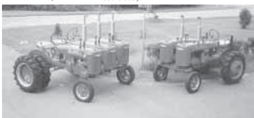
Tractor runs on one, two or three engines in any order. It has two steering wheels and two sets of clutch and brake pedals so Stewart can drive the tractor from either side.
