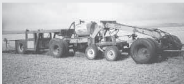
The "Gadget" is a 77-ft. long rig equipped with 17 tires and a 14,000-lb. packer on back. Machine's center section has four large tires that can be raised and lowered to pre-form the soil into a hump.
