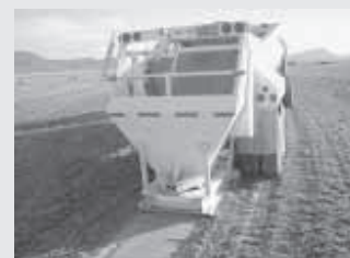
Hydraulic-operated door at back of trailer has a steel compactor plate underneath it.
