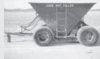
Agee's original center pivot rut filler has duals all the way around and lowers to the ground to fill ruts.
