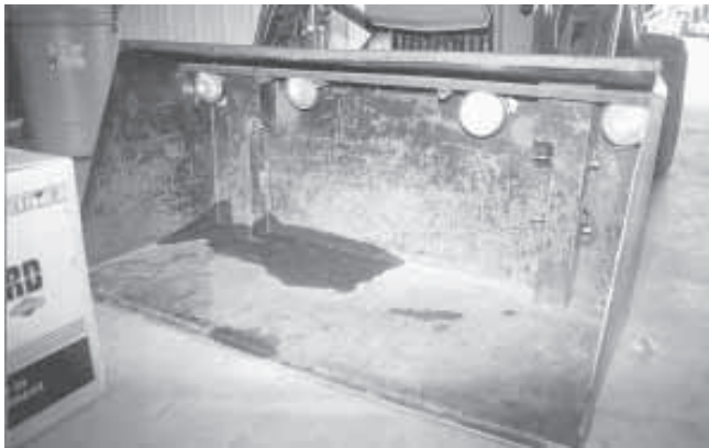
Bucket-mounted lights automatically tilt up and down with bucket, so they shine exactly where the light is needed.
