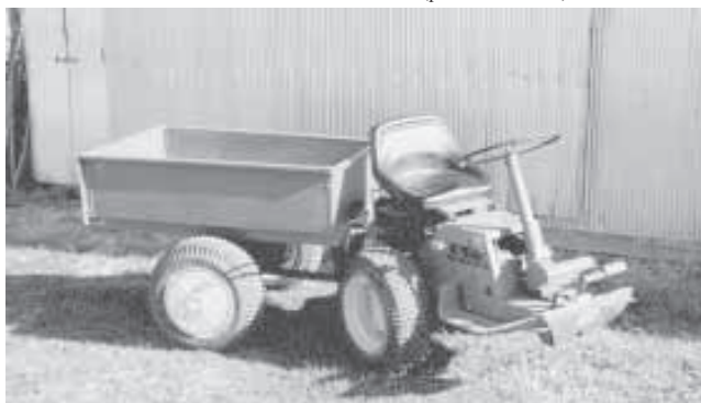
To make his utility vehicle, Stanley Byerly joined a dumping yard trailer to an old Deere 72 front deck riding mower.
