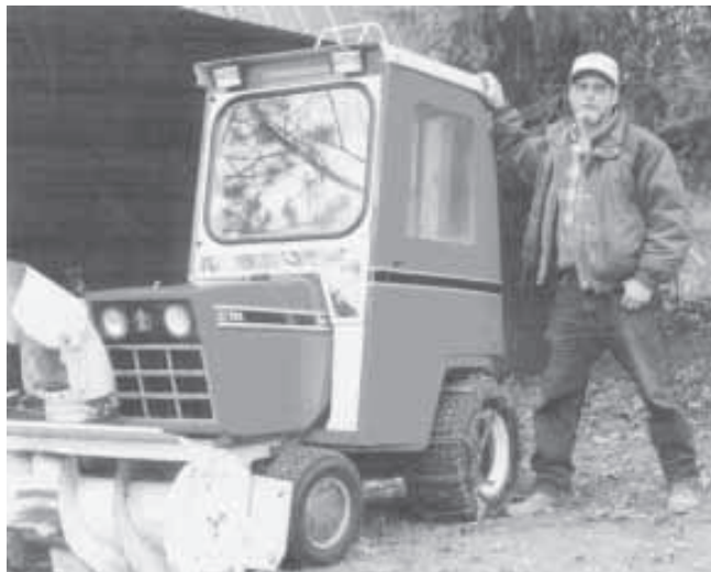
Biech's home-built cab has a hinged glass windshield that lets him easily check engine fluids. Hinge pins pull out so he can remove windshield.
