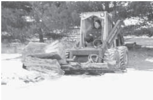
Unit can split logs up to 46 in. long and any diameter.
