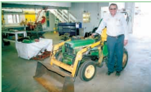
This 1973 Deere Hydro 140 equipped with a front-end loader was originally equipped with a Kohler 14 hp engine. Kaczmarek replaced it with a 14 hp Vanguard.
