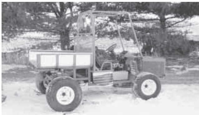
David Miller started with a 1987 Subaru Brat 4-WD pickup and ended up with a utility vehicle. "I use it for hauling rocks, dirt and wood, pulling wagons, and so on," he says.
