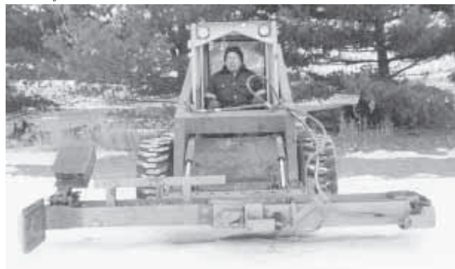
Splitter consists of a 10-ft. long, steel I-beam with a fixed push plate at one end.
