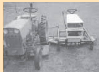
Davis pulls the wing mower alongside his Power King garden tractor, which has a 4-ft. deck. Four caster wheels allow the wing mower to move in any direction with the Power King.
