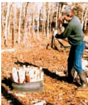
Bokenfohr uses a cut-down tire to hold a bunch of wood blocks to split all at once.
