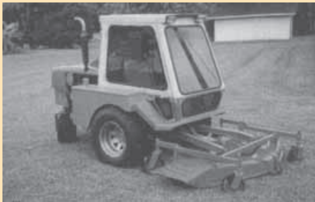
Robert Judice built this zero turn riding mower. It has an air conditioned cab and a 5-ft. deck that automatically raises or lowers according to mowing conditions.
