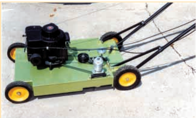
"It lets me mow my lawn without leaving a thin strip of grass next to building foundations, etc.," says Marty Garrett about the trimmer he added to the left side of his mower.
