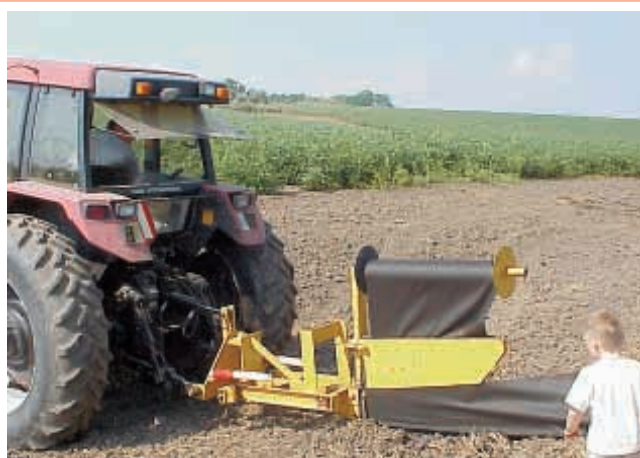
New 3-pt. mounted fabric layer is equipped with a single large shank with a roll of fabric on a horizontal shaft above it.
