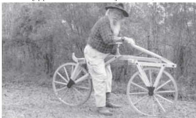
Chuck Smart built this replica of the first bicycle ever built. It has no pedals. You just run and coast.
