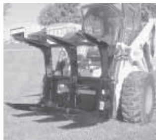
Grapple fork can be used to break up concrete much faster than a jackhammer or other conventional methods.
