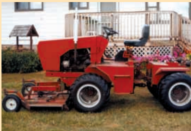
Using mostly junked parts, Harold Tribitt built this 4-WD articulated "mower tractor" equipped with a 6-ft. front-mounted deck that rides on a pair of caster wheels.
