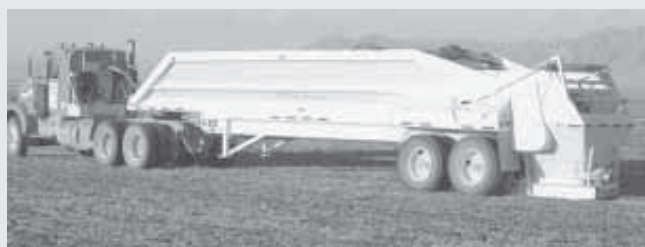
Jace Agee recently built this 10-wheel semi trailer rut filler. It holds 22 yards of material and can travel at highway speeds.
