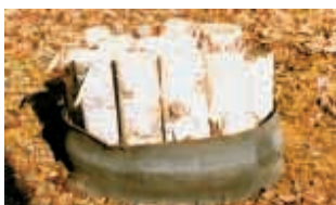
Bokenfohr uses a cut-down tire to hold a bunch of wood blocks to split all at once.
